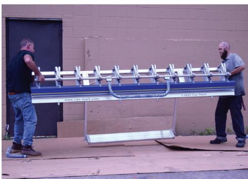
Use two people to lift brake and set up in normal operating position and pivot walk board at front of stand into flat position.
