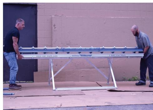
From the rear of the brake, remove fast pins from rear struts on base rails of brake and lower struts to meet rear legs of extreme stand. Insert fast pins to secure struts in place.
